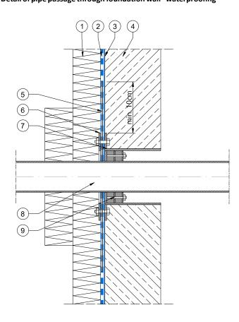
**NOTE:** Adjust the thickness of the waterproofing layers to the existing soil and water conditions
